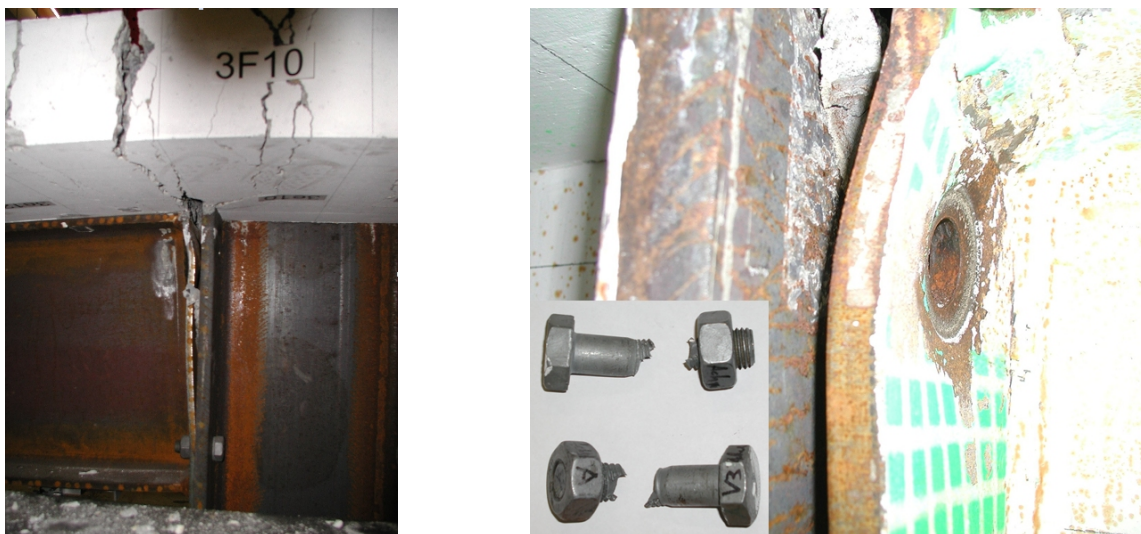
Figure 4-71: Unexpected brittle bolt failure in previous test conducted in Stuttgart [83]
