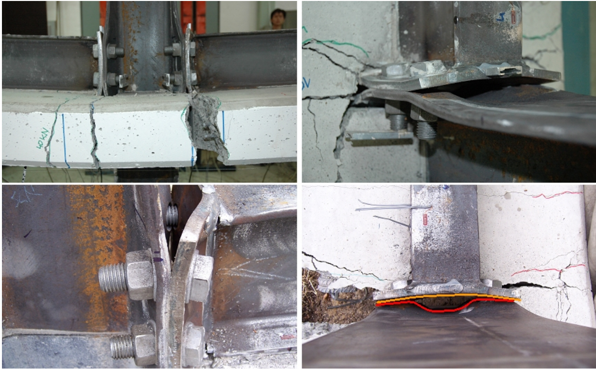
Figure 4-63: Test specimen V1 after failure under M-N exposure (hogging)
