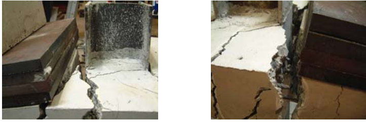
Figure 4-33: Collapse of the longitudinal rebars in the vicinity of the external composite joints at point “D” of Figure 4.31
