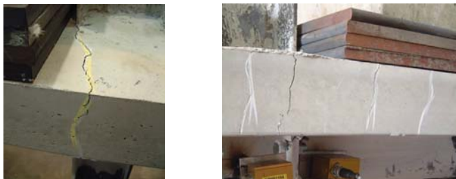
Figure 4-29: Accentuated cracks in the vicinity of the external composite joints at the formation of the beam plastic mechanism
