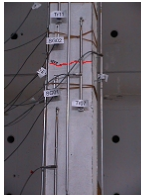
Figure 4-93: Crack path for specimen RCRR
