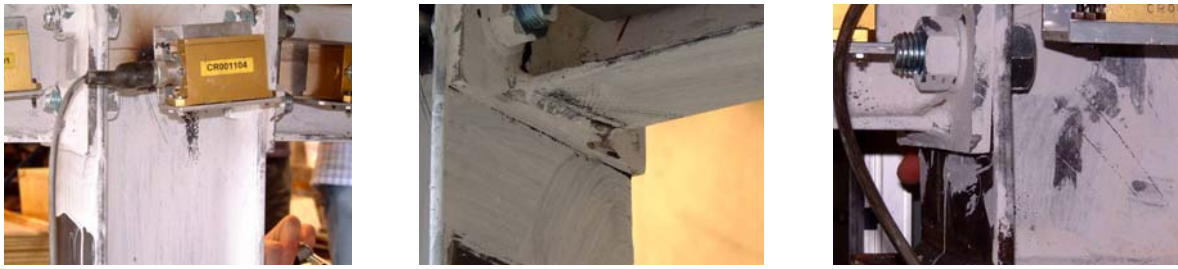
Figure 4-30: Yielding of steel component at the external and internal composite joints
