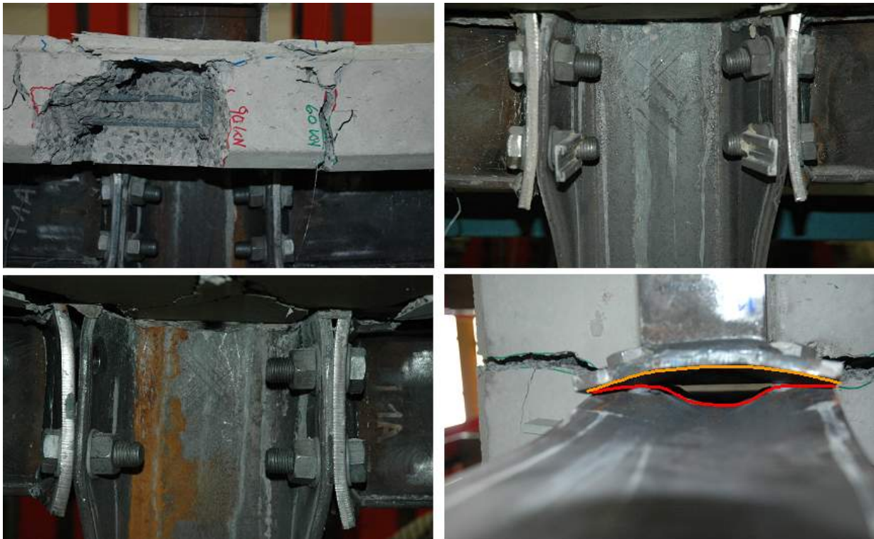
Figure 4-64: Test specimen V4 after failure under M-N exposure (sagging)
