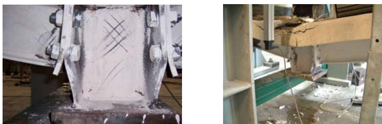
Figure 4-38: Internal composite joints at the end of the test
