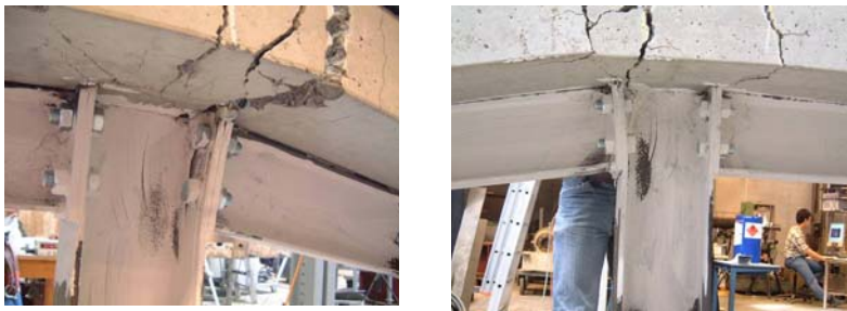
Figure 4-34: Yielding spread in the steel components of the external composite joints
