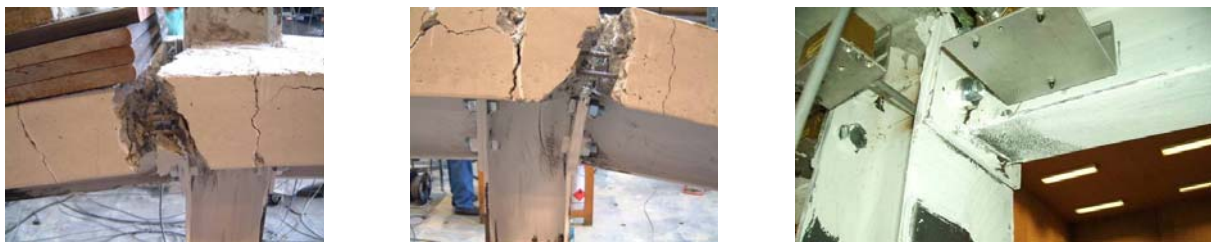
Figure 4-37: External composite joints at the end of the test
