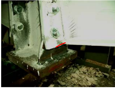
Figure 4-39: Cracks in the welds between the IPE140 profile and the end-plate
