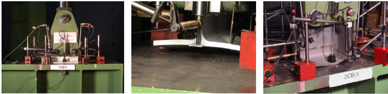
Figure 4-101: Typical transducers' set-up for tension tests on T-stubs.
