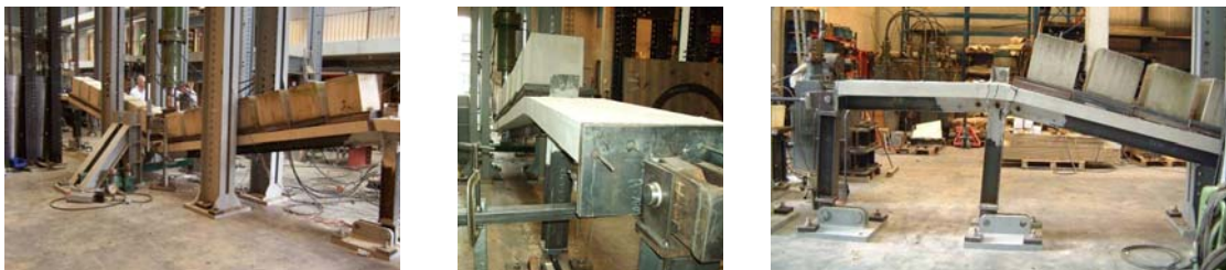
Figure 4-36: Deformation of the specimen at point “E” of Figure 4-28 and horizontal displacement of the specimen at point “E” of Figure 4-28
