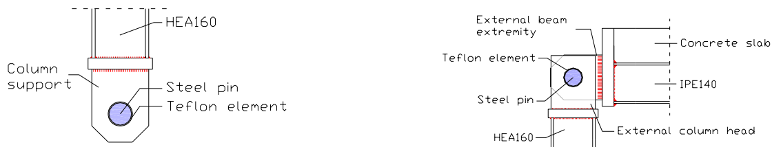
Figure 4-16: Column support and hinge at the external joints
