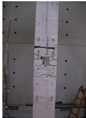
Figure 4-92: Crack path for specimen RCSL
