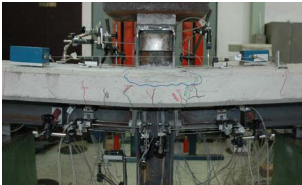
Figure 4-58: Crack distribution and deformation behaviour for sagging moment
