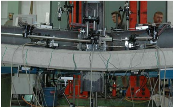
Figure 4-55: Crack distribution in the distance of the stirrups
