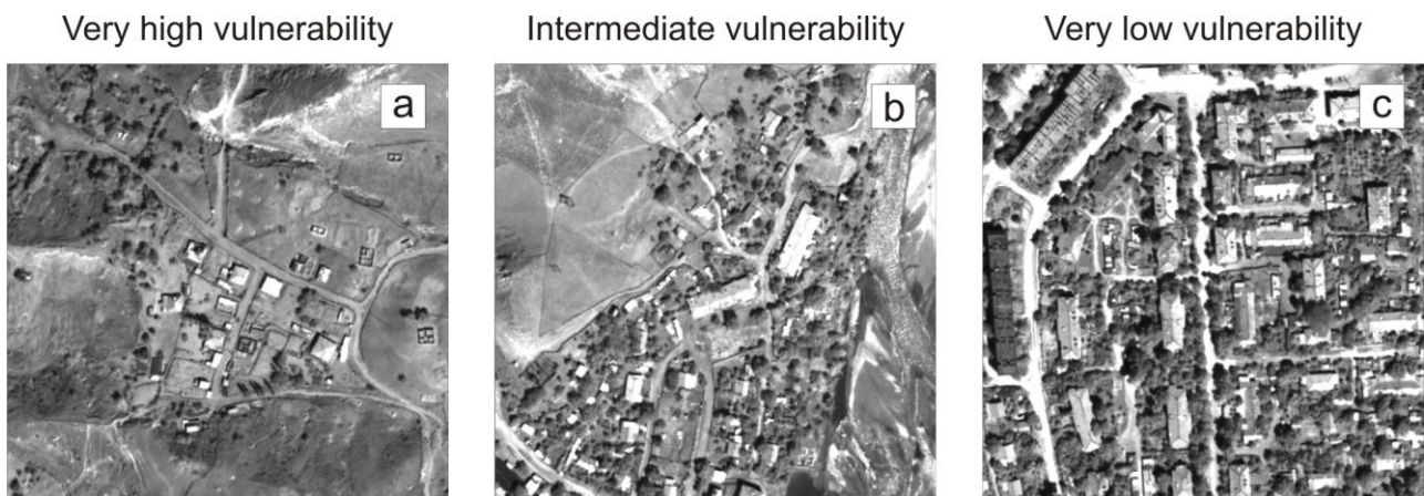
Figure AF.87: Snapshots of the 2007 Quickbird imagery showing clusters of inhabited area with very high (a), moderate (b) and very low (c) vulnerability, assigned based on the interpreted proportion between two building types.
