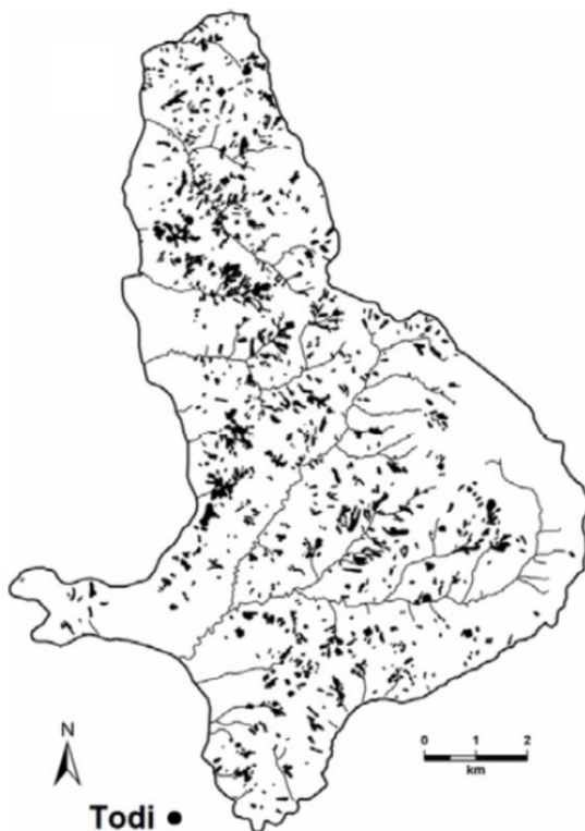
Figure AF.7: Landslide inventory and landslide susceptibility maps for Collazzone study area, Italy (landslide susceptibility is mapped by the DA method - by Guzzetti, 2006).
