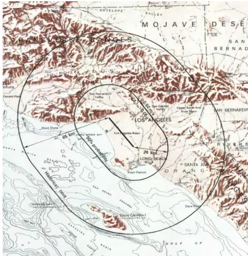
Figure BF.3: An example of the landslide susceptibility mapping performed by Wilson and Keefer (1985) - the external outline shows the maximum landslide occurrence zone and the inner outlines denotes 50% occurrence probability zone (by Wilson and Keefer, 1985).
