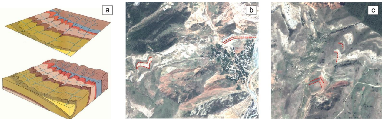
Figure AF.53: (a) Schematic representation of roughly parallel outcrop patterns in a cataclinal slope (by Dirik, 2005); (b) and (c) sample views from above at the V-shape structures in the target area (the Quickbird imagery, Google Earth software).
