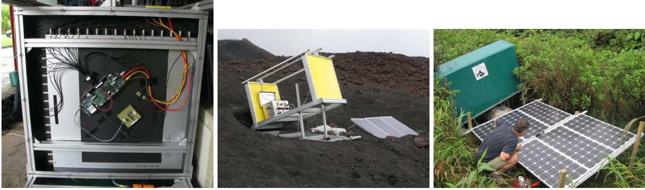
Figure 10: Left: matrix with open case. Middle: complete telescope at the summit of Mount Etna in Sicily. The dip is 30^\circ and the distance between the two matrices is of 115 cm. Solar conditions there allow single solar unit use. Right: telescope covered with its tarpaulin on La Soufrière of Guadeloupe. Two solar units of 270 W each are mandatory because of cloudy weather.
