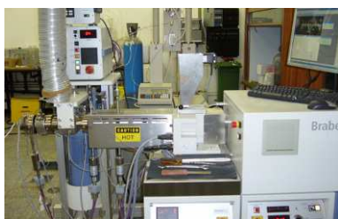
Fig.4: Single-screw extruder designed for supercritical fluid injection, used for continuous polymer foaming.
