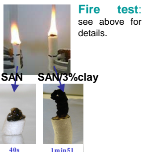
Fig.6: Qualitative fire tests performed with SAN and SAN/clay nanocomposite foams.
