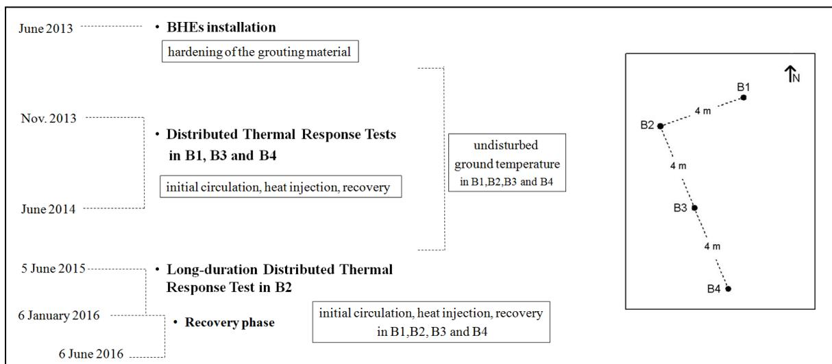
Figure 2 - In-situ temperature measurements in the four BHEs (B1-B4) (June 2013 - June 2016)
