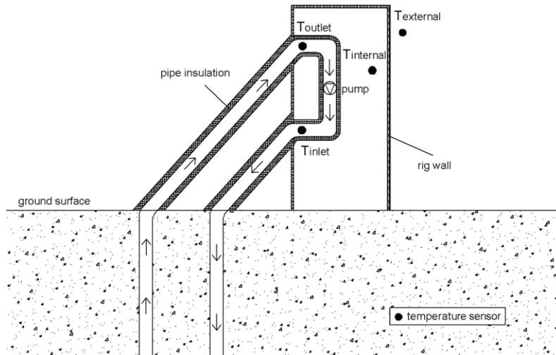
Figure 3 - Temperature sensors location during the DTRTs
