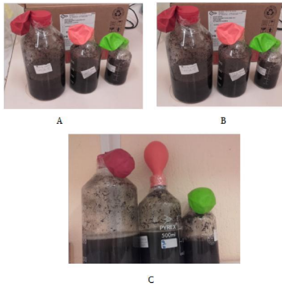
Figura 3. Experiments conducted with bottles balloon, A) the first day of the experiment, B) as anaerobic conditions were set for 24 hours, and C) observation of biogas production.
