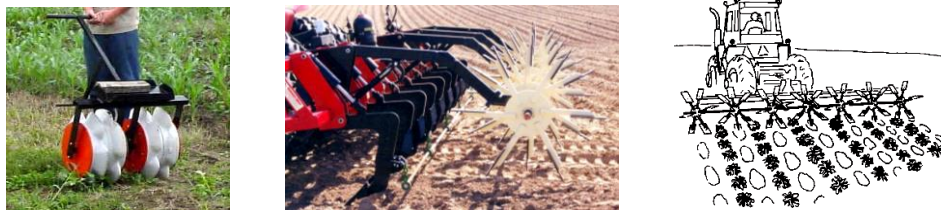
Figure 8. A hand type soil conditioner and a combination of inter-row ripper and multi-spoke “spider” (Geisel, 2012; Keith, 2016; http://www.Terramanustech.com ; http://www.dammerdiker.com )
