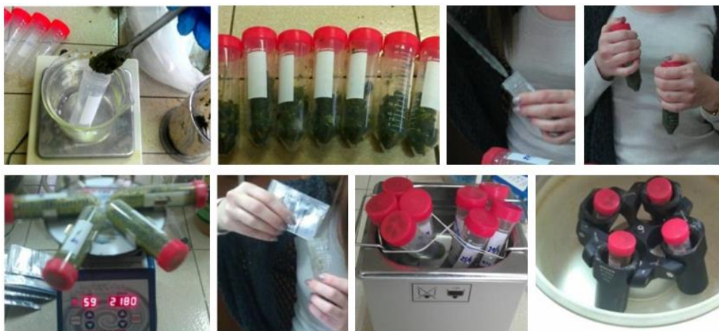
Figure 1. The procedure of cyprodinil and fludioxonil extraction from lettuce
