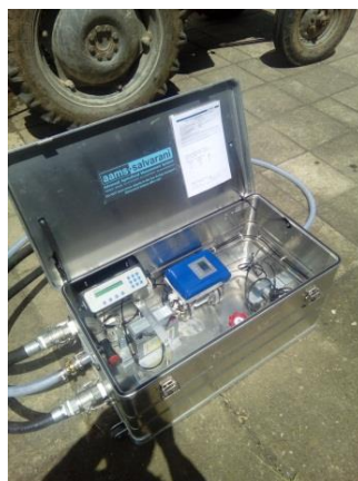
Figure 2. Pumptester and flowmeter- AAMS-SALVARANI
