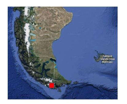
A wind farm in the southern part of South America can generate 13 W/m², against 3 W/m² in mainland Europe. The total consumption of electricity in Brazil, which is around 500 TWh/year, could be generated by covering the red area on this map with wind mills.
