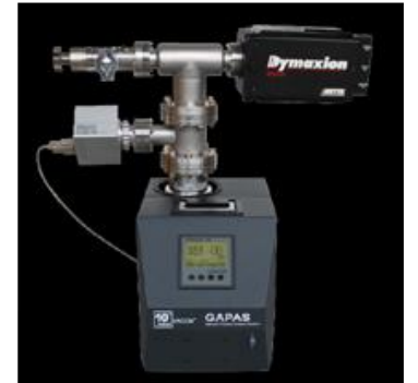
Membran-inlet Mass spectrometry MIMS (e.g. Vacum, Pfeiffer)
