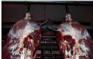
Picture 2: position of probes for the measurement of core temperature
