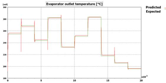
Figure 1: Example of comparison against steady-state model for an evaporator using ethanol.
