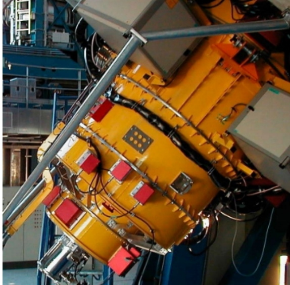
Figure 2.5: FORS2 instrument at the Cassegrain focus of the VLT UT1 (Antu). Credit ESO.
