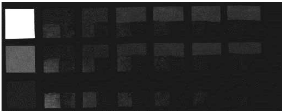
Fig. 6 – VIL, digital overexposure. Lines of samples based on EB, CR and CY as drugging pigments.
