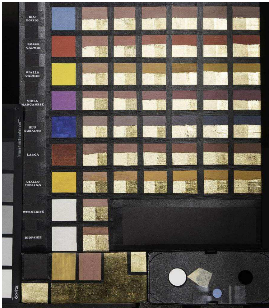
Fig. 3 – Set of samples (3 cm high per 3.5 cm wide). Drugging pigments (EB, CR, CY, MV, CB, LD, IY, WE, DI) along the first column. Along the lines: bole mixtures prepared with 2%, 5%, 10%, 15%, 20% and 25% in weight of the drugging pigment on the left, and with 33% in weight of WE and DI, where the lower part is covered by the gold leaf and only the half on the right is burnished. On the bottom: references for the study (the reddish one is the bole reference ; the gilding reference is the bigger “upside down T” area).
