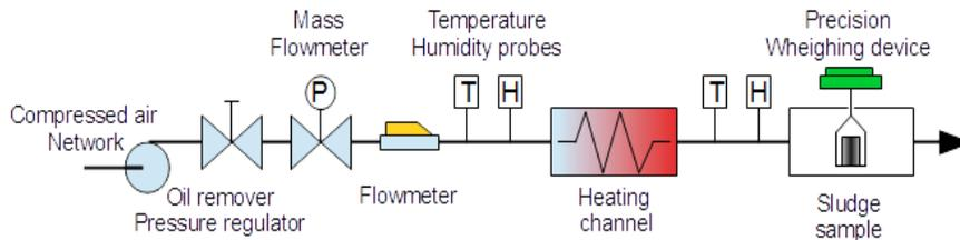
Figure 2: Scheme of the convective micro-dryer.
