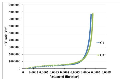
Fig. 4. Dewatering curves of central point's CT
