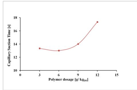
Fig. 3. CST results on activated sludge
