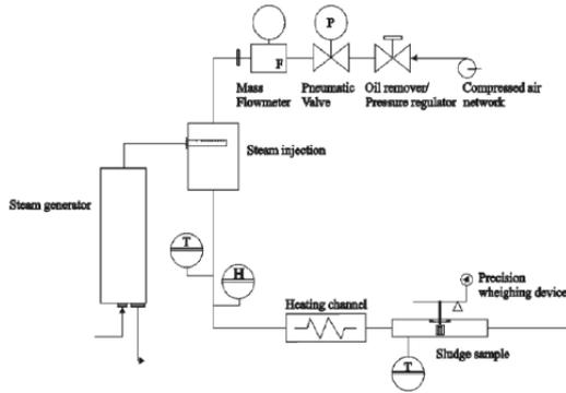
Fig. 2. Scheme of the convective micro-dryer.
