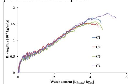
Fig. 6c. Krisher's curves of central point's CT Repeatability test
