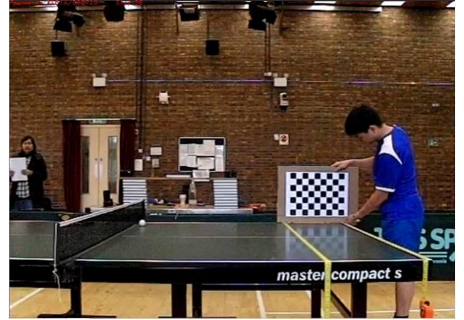
Figure 4 A double-sided checker board used for calibration
