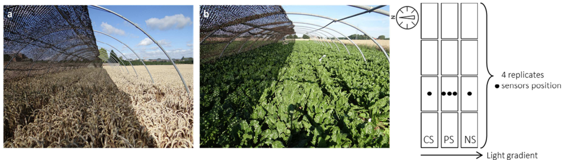
Figure 1: Artificial shade structure above winter wheat (a) and sugar beet (b). The right frame corresponds to the general lay out of the experimental device : the three modalities (CS, PS, NS) and the light sensors position located along a north-south gradient.
