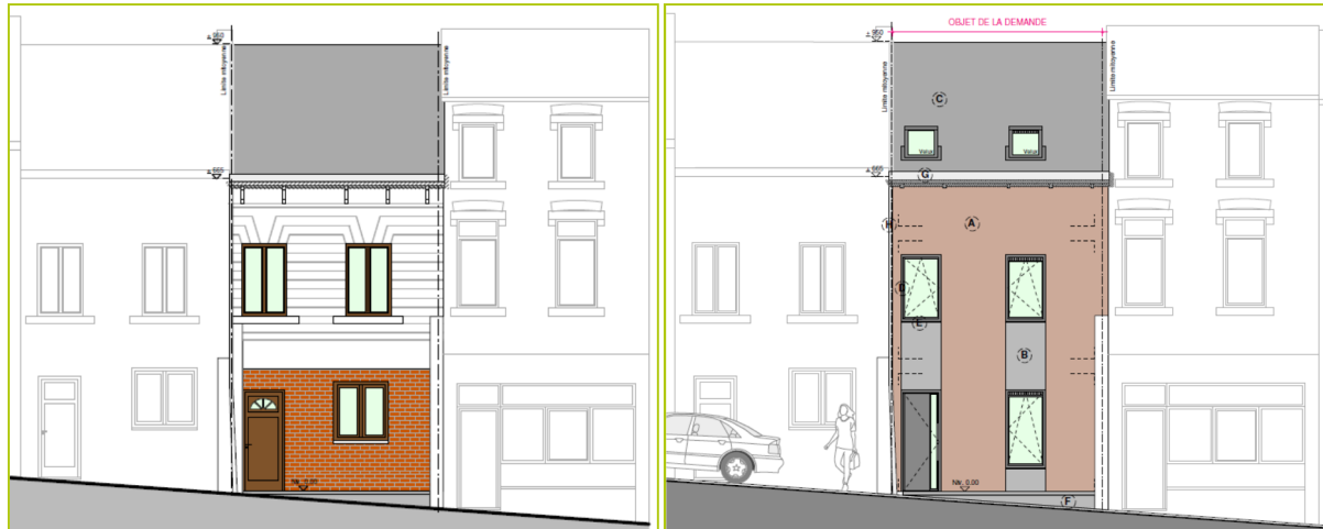
Figure 2. Front facade of the renovated building, before (left) and after (right) renovation.
