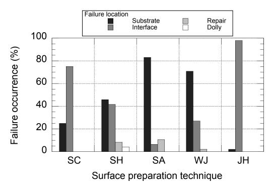
Figure 3-26: Distribution of failure location in pull-off tests performed on 30-MPa substrates after repair (UL program)
