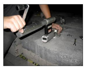
Figure 0-4: Pull-off bond test apparatus
