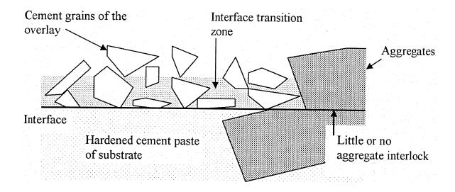
Figure 1-2: Weak zone between substrate and repair system [7]
