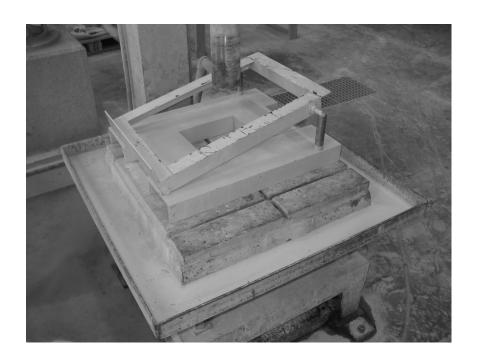
Figure 0-7: Special device for controlling the coring axis inclination at U. of Liège
