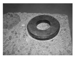
Figure 5-3: Gluing of the ring onto the concrete substrate (ISAT)
