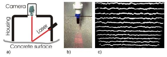
Figure 2-7: Laser profilometry – a) schematic representation of the laser profiling testing device; b) line laser; c) laser image of a concrete surface
