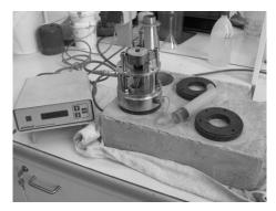
Figure 5-2: Autoclam system and electronic controller
