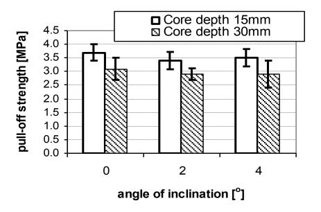
Figure 0-8: Average pull-off strength values for concrete slabs C30/37
