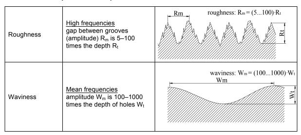
In accordance with EN ISO 4287, the total (primary) profile, the waviness and roughness profiles can be characterized by several vertical (Table 2-3) and horizontal (Table 2-4) amplitude parameters. Surface parameters are determined on the basis of the mean line as a reference line: this reference is usually defined in such a way that, in the limits of the profile length, the sum of the squared values of the altitudes of the profile measured versus this reference line is minimal.
