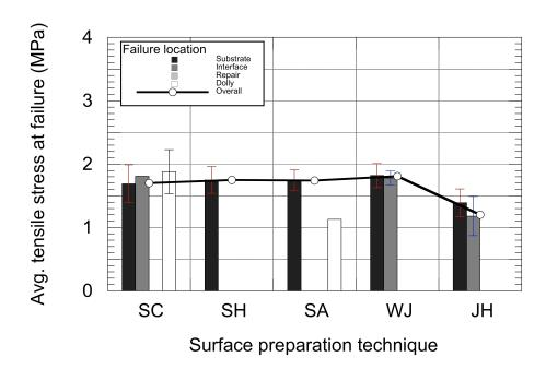
Figure 3-23: Results of pull-off tests performed on 20-MPa substrates after repair (UL program)
