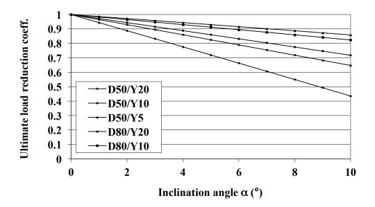
Figure 0-2: Effect of the angle, the core depth and diameter on ultimate load reduction coefficient
