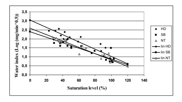
Figure 5-13: Permeability index versus degree of saturation (ISAT) after elimination of extreme values
