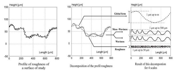
Figure 2-8: Effect of scale on profile decomposition
