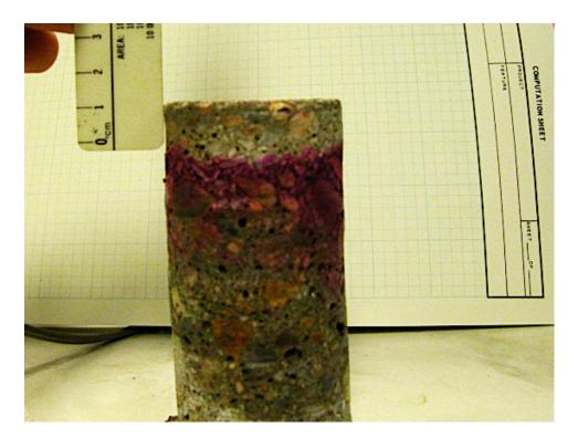
Figure 0-2: Carbonation depth measurement on a freshly exposed concrete section using phenolphthalein
