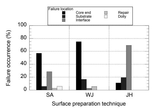
Figure 3-12: Distribution of failure location in pull-off tests performed on 40-MPa substrates after repair (USBR program)
