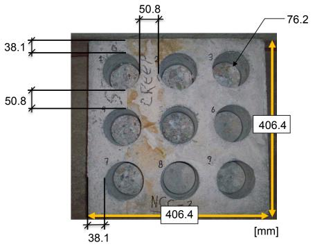
Figure 0-3: Slab coring template
