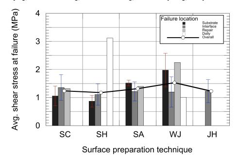
Figure 3-27:Results of torque tests performed on 20-MPa substrates after repair (UL program)
