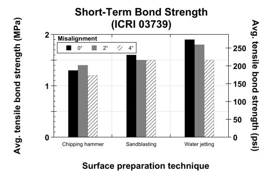
Figure 0-12: Average pull-off test results - repaired substrates
