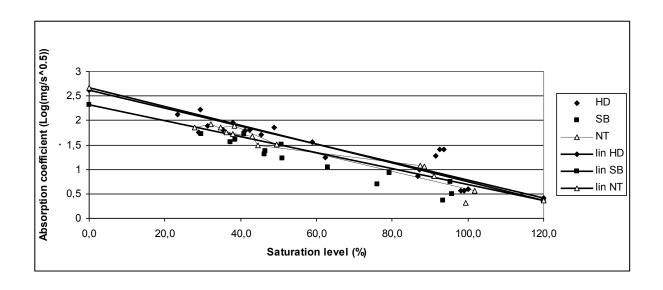
Figure 5-11: Capillary absorption rate versus degree of saturation (MCST)
