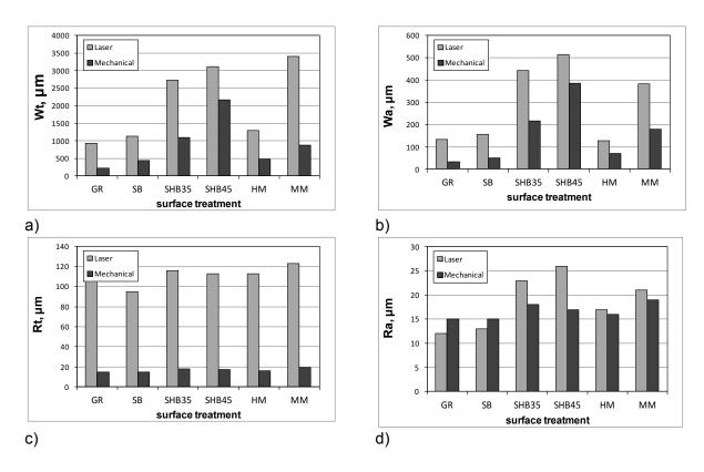
Figure 2-13: Waviness parameters a)  $W_t$  and b)  $W_a$ ; microroughness parameters c)  $R_t$  and d)  $R_a$ ; as determined through laser and mechanical profilometry
