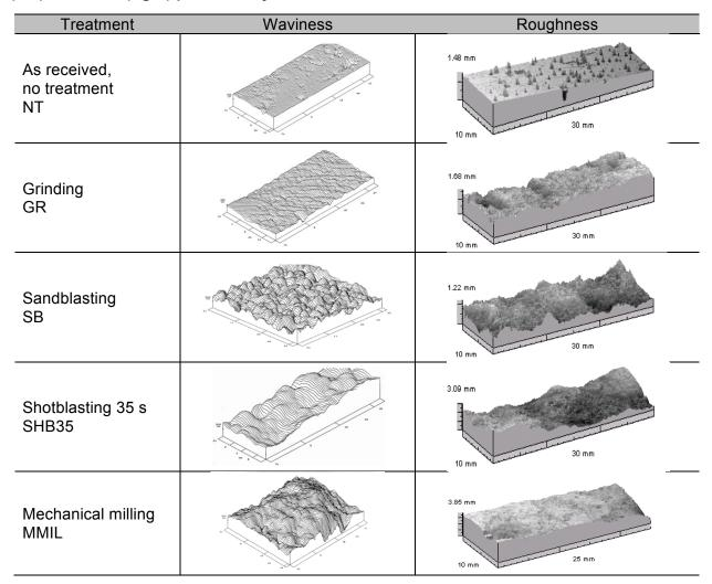
The results of surface geometry characterization with the four methods can be summarized as illustrated in Figure 2-13. The geometrical parameters determined for the microscopic level (profile amplitude parameters) generally indicate that the highest roughness was obtained for shotblasting after 45 seconds and the lowest for grinding (Figure 2-13). With respect to profilometry methods, the waviness parameters are lower than those of the total profile by about
