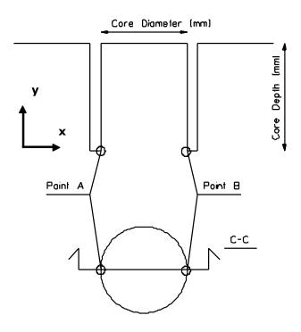
Figure 0-4: Pull-off geometry considered in the numerical analysis
