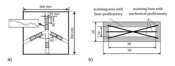
Figure 2-10: Illustration of a) sampling for microscopic observation; and b) surface geometry characterization with laser and mechanical profilometry
