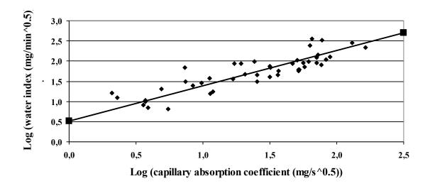
Figure 5-12: Comparison between permeability index and capillary absorption
