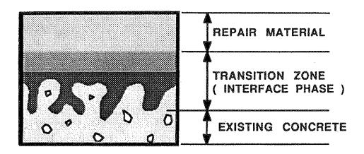
Figure 1-3: Idealized model of a surface repair system [8]
