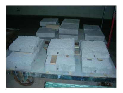
Figure 0-1: Base slabs after surface preparation
