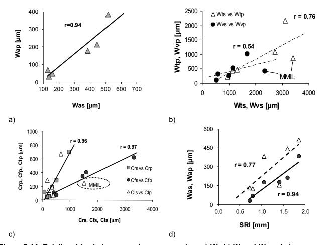
Figure 2-14: Relationships between waviness parameters a)  $W_a$ , b)  $W_t$  and  $W_v$  and c) Abbott parameters, determined through laser ( $\Delta$ ) and mechanical (•) profilometry; d) relationship of  $W_{as}$  and  $W_{ap}$  vs. SRI
