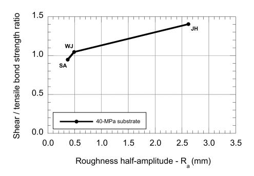
Figure 3-20: Shear bond to tensile bond strength ratio after repair as a function of the substrate R<sub>a</sub> value generated by various preparation techniques (USBR program) (note: SA – sandblasting; WJ – water jetting; JH – jackhammering)
