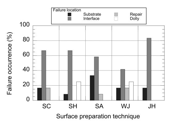
Figure 3-30: Distribution of failure location in torque tests performed on 30-MPa substrates after repair (UL program) (note: SC - scarifying; SH - shotblasting; SA - sandblasting; WJ - water jetting; JH - jackhammering)
