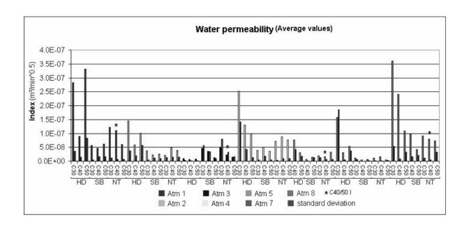
Figure 5-8: Permeability index for the different conditions: concretes, storage conditions (atm) and surface preparation.
