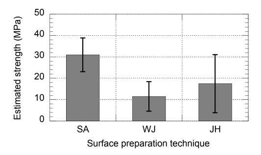
Figure 3-10: Results of Schmidt hammer soundings (ASTM C805) performed after surface preparation to evaluate the mechanical integrity of the exposed concrete surface (USBR program)
