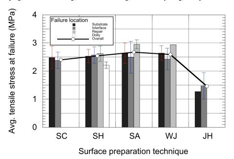
Figure 3-25:Results of pull-off tests performed on 30-MPa substrates after repair (UL program)
