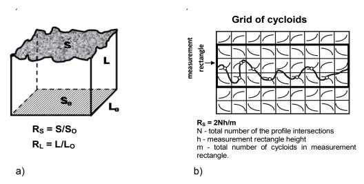
Figure 2-11: a) Significance of the  $R_S$  and  $R_L$  parameters; b) evaluation of the  $R_S$  value using grid of cycloids
