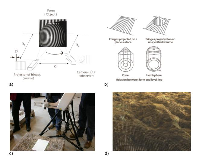
Figure 2-6: Optomorphological profilometry – a) principle of measurement; b) relationship between form and level line; c) testing equipment; d) example of 3D representation of concrete surface (University of Liège)
