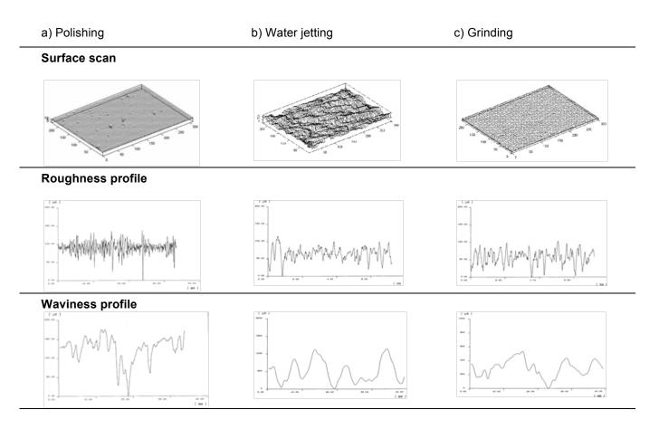
Figure 2-17: 3D representation of surfaces and corresponding roughness and waviness profiles for three different types of treatment
