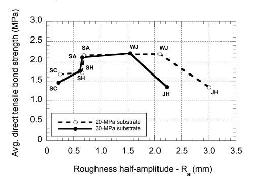
Figure 3-32: Results of direct tensile tests (CRD-C 164) performed after repair on cores extracted from the slabs as a function of the substrate roughness generated by various preparation techniques (UL program) (note: SC – scarifying; SH – shotblasting; SA – sandblasting; WJ – water jetting; JH – jackhammering)
