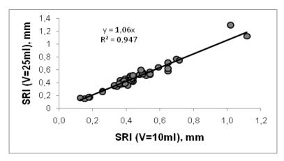
Figure 2-12: Influence of the sand volume used in the sand patch test
