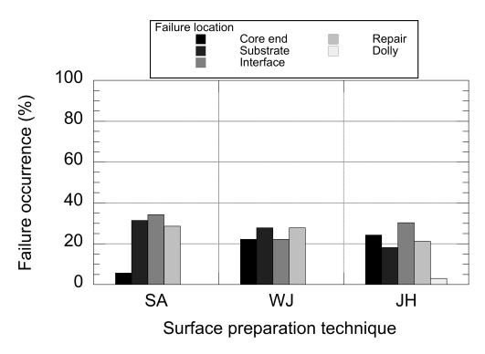
Figure 3-14: Distribution of failure location in torque tests performed on 40-MPa substrates after repair (USBR program)
