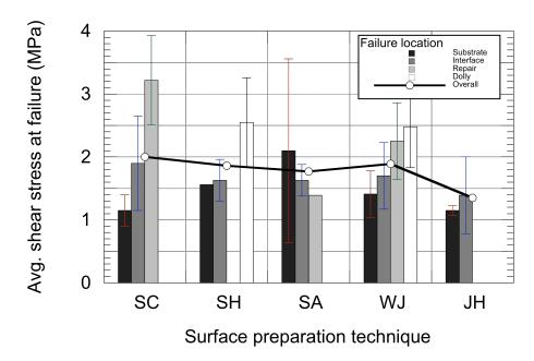
Figure 3-29: Results of torque tests performed on 30-MPa substrates after repair (UL program)
