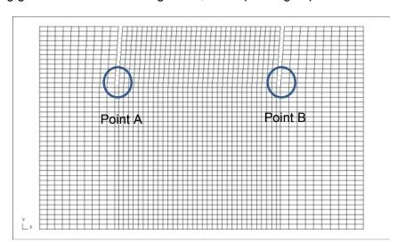
Figure 0-3: FEM mesh for Pull-off simulation (4° coring angle and 30 mm coring depth)
