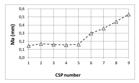
Figure 2-19: ICRI CSP evaluation (Guideline No. 310.2R–2013) – a) photographs of the nine replicates ordered from 1 to 9; b) characterization of the CSP replicates performed by Perez et al. using an interferometric method [5]
