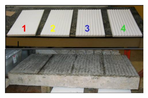
Figure 3-6: V-shape rippled acrylic dies and resulting profiled slabs (UL program)
