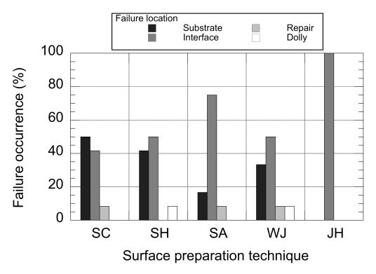
Figure 3-28: Distribution of failure location in torque tests performed on 20-MPa substrates after repair (UL program)
