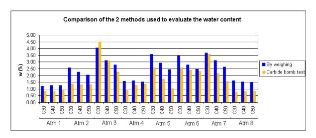
Figure 5-7: Comparison of water content of concrete samples obtained with specimen weight method and *Carbide bomb* test method
