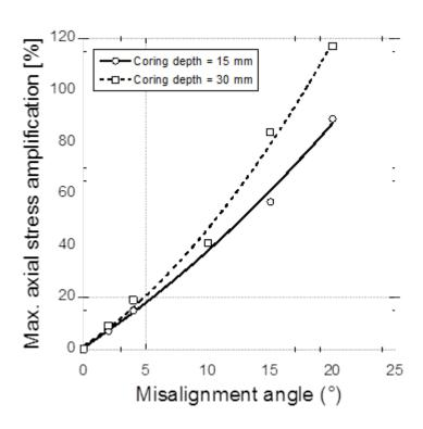
Figure 0-6: Theoretical axial stress ( $\sigma_y$ ) amplification as a function of the misalignment angle of inclination and coring depth in a pull-off experiment.
