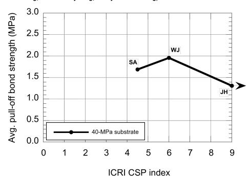
Figure 3-15: Results of pull-off tests (ASTM C1583) performed after repair as a function of the substrate CSP index (ICRI No. 310.2R-2013) generated by various preparation techniques (USBR program)
