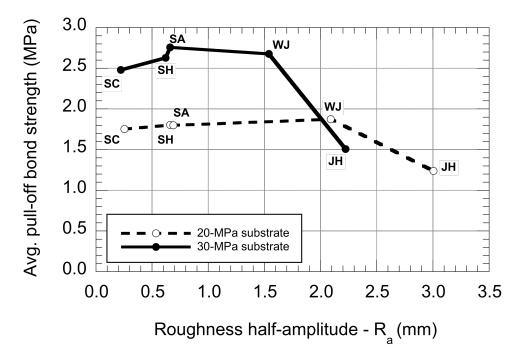
Figure 3-31: Results of pull-off tests (ASTM C1583) performed after repair as a function of the substrate roughness generated by various preparation techniques (UL program) (note: SC - scarifying; SH - shotblasting; SA - sandblasting; WJ - water jetting; JH - jackhammering)
