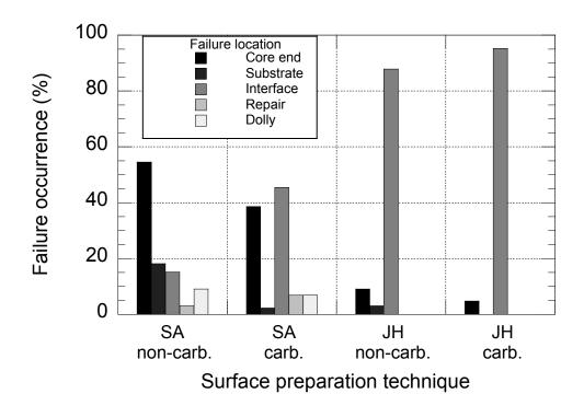
Figure 0-6: Bond strength results for the sandblast surface preparation
