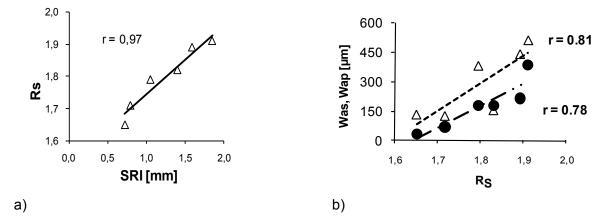
Figure 2-15: Relationships a)  $R_S$  vs. SRI and b)  $R_S$  vs. arithmetic mean deviation of waviness profile, as determined through laser ( $W_{as}$ ) and mechanical ( $W_{ap}$ ) profilometry
