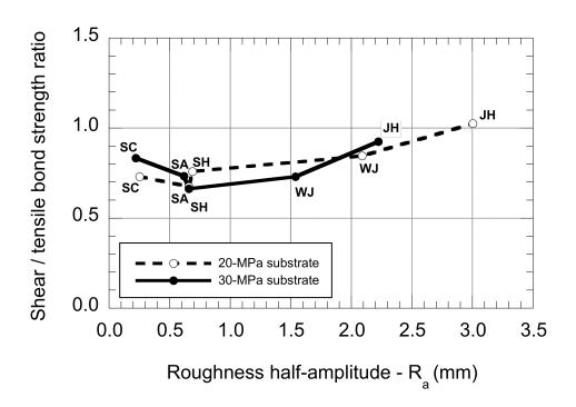
Figure 3-35: Shear bond to tensile bond strength ratio after repair as a function of the substrate R<sub>a</sub> value generated by various preparation techniques (UL program) (note: SC – scarifying; SH – shotblasting; SA – sandblasting; WJ – water jetting; JH – jackhammering)
