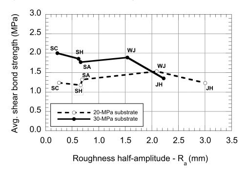
Figure 3-34: Results of torsional bond experiments performed after repair as a function of the substrate roughness generated by various preparation techniques (UL program) (note: SC – scarifying; SH – shotblasting; SA – sandblasting; WJ – water jetting; JH – jackhammering)
