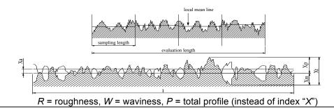
Table 2-4: Horizontal amplitude parameters of surface profile as per EN ISO 4287
