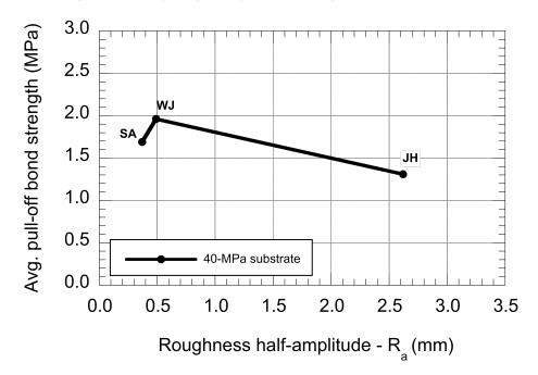
Figure 3-17: Results of pull-off tests (ASTM C1583) performed after repair as a function of the substrate R<sub>a</sub> value generated by various preparation techniques (USBR program) (note: SA – sandblasting; WJ – water jetting; JH – jackhammering)
