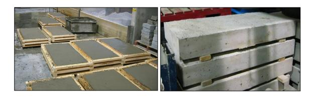
Figure 3-4: Test slabs prepared at UL
