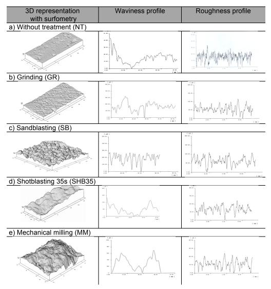
Figure 2-3: Examples of 3D representation with surfometry, waviness and roughness profiles after different surface treatments, as determined through mechanical profilometry (University of Liège)
