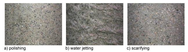
Figure 2-16: Concrete surface profiles obtained with selected surface preparation methods
