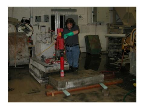
Figure 0-10: Experimental setup for coring under controlled inclination at USBR
