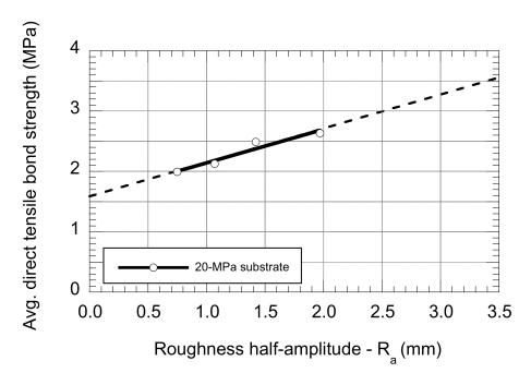
Figure 3-33: Results of direct tensile tests performed after repair on cores extracted from the artificially profiled 20-MPa test slab (UL program)
