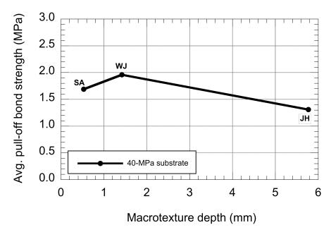
Figure 3-16: Results of pull-off tests (ASTM C1583) performed after repair as a function of the substrate Macrotexture depth (ASTM E965) generated by various preparation techniques (USBR program)
