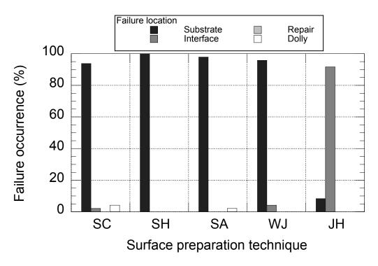
Figure 3-24: Distribution of failure location in pull-off tests performed on 20-MPa substrates after repair (UL program)
