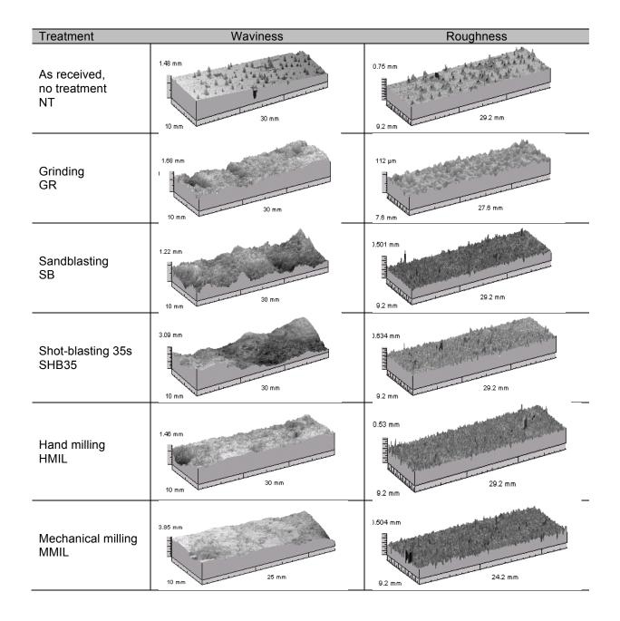
Figure 2-5: Examples of 3D representation of specimen surfaces obtained by laser profilometry after waviness and roughness filtering
