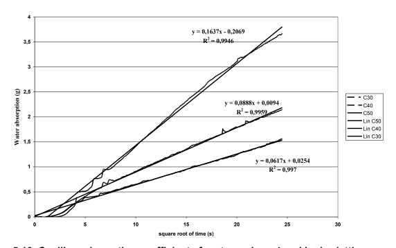
Figure 5-10: Capillary absorption coefficients for atmosphere 4 and hydro-jetting
