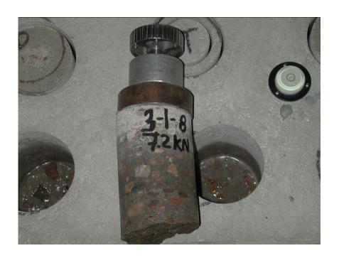
Figure 0-11: View of a 4°-inclined core after pull-off extraction
