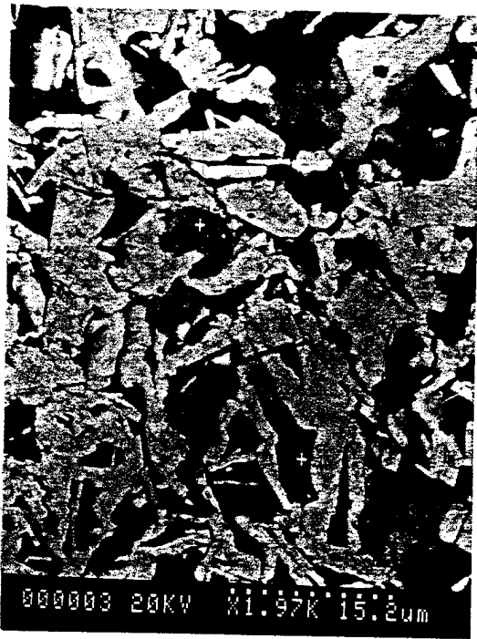
FIG. 1. Micrographs showing microscopic impurities incorporated in the main phase (indicated by a cross).
