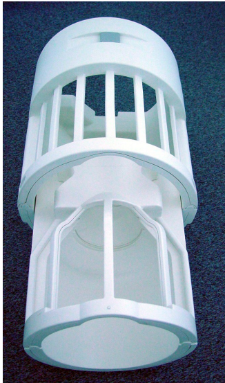
Figure 4.3: Tx/Rx coil for ^{17}\text{O} at 9.4 T.
