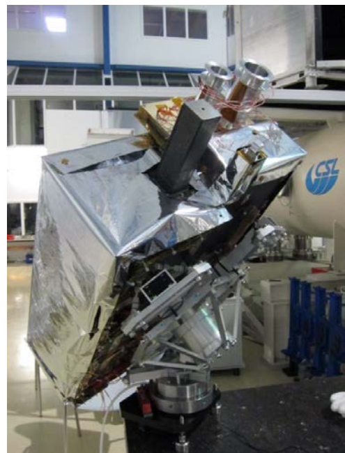
Figure 6 – EUI OBS STM MoI and CoG measurement
