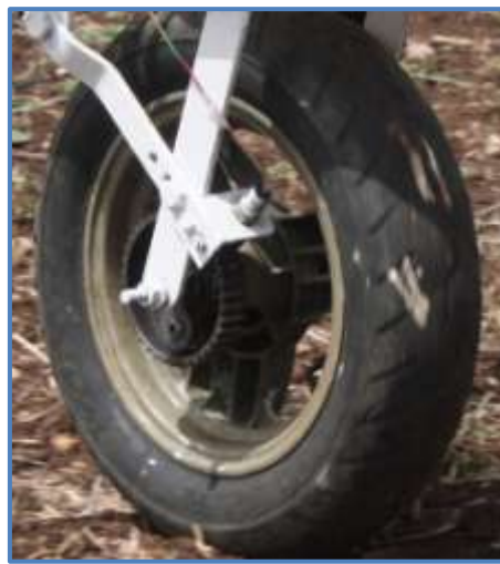
Figure 44: Design of a gear of 38 square teeth mounted on a wheel circumference of 1.2 m for sensing speed of the DIS sprayer chariot
