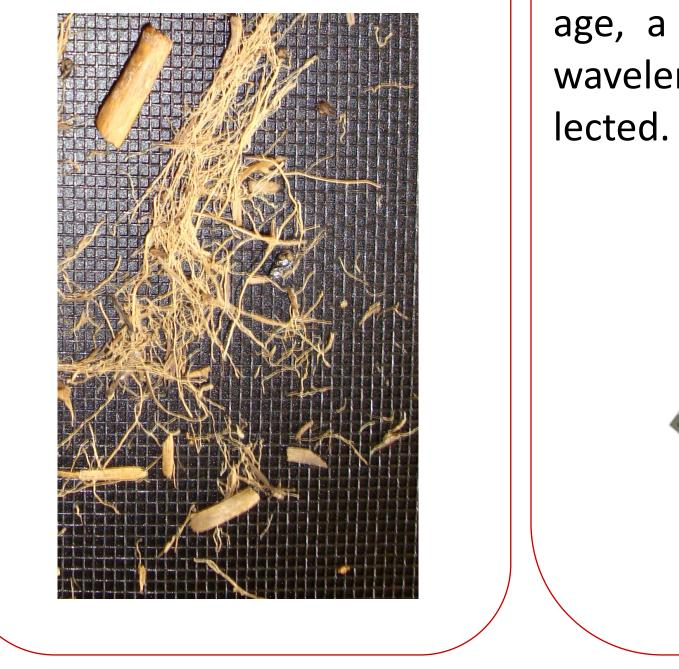
NIR images were acquired with a **NIR hyperspectral line scan** (= push-broom) (Vermeulen et al., 2012). Samples were laid on a conveyor belt placed under the NIR camera. For each pixel of the NIR image, a complete spectrum including 209 wavelengths (1100-2498 nm) was colA dichotomist classification tree based on 3 successive PLS or SVM models was used to separate spectra into 4 distinct classes: background, soil, crop residues and roots (Eylenbosch et al., 2014; Fernández Pierna et al., 2004).
