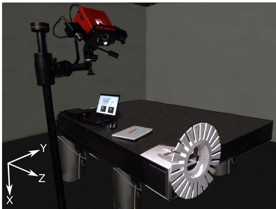
Figure 5.2: Test set-up for the optical measurement of the geometry.
