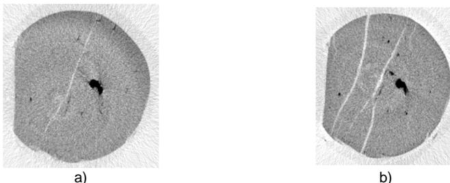
Figure 1: Cross-sections of a clay sample around 13 mm in initial diameter before and after complete dessication. The noise level is high because the experiment was not made in-situ so the sample had to spend the least amount of time out of the drier. In this sample a nick was made on the left side to adjust its position for the scan.
