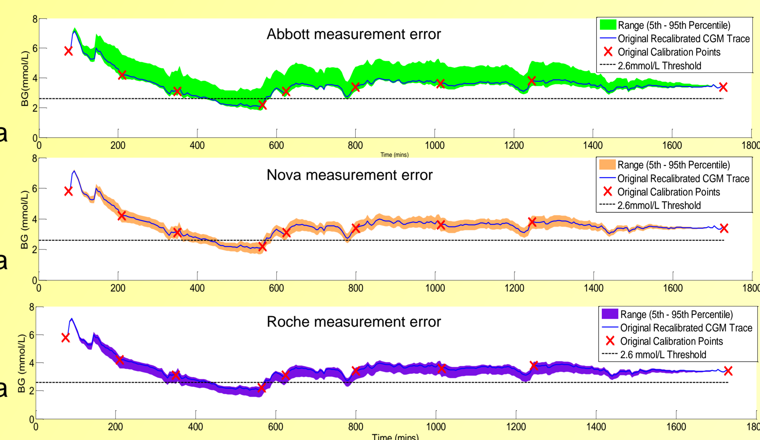
Figure 3: CGM traces showing the effect of Abbott measurement error (top), Nova measurement error (middle), and, Roche measurement error (bottom). The colored band in each plot shows the 5 th -95 th percentile range in CGM data over 1000MC simulations.
