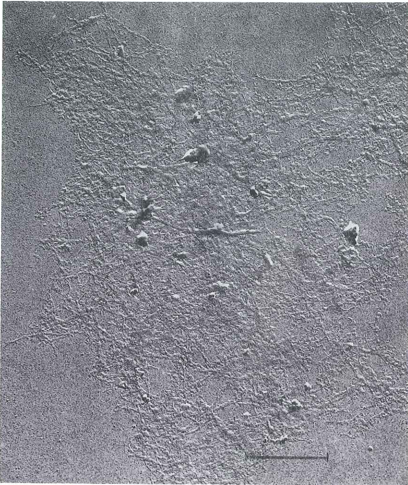
Fig. 11. Microfibrils of nacreine (mother-of-pearl of Nautilus shell), after decalcification and treatment by NaOH 0.5 N at 100° during 13 h. After Goffinet 149 . Scale = 1 \mu .
