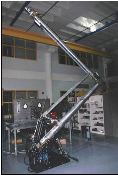
Figure 12: Ralf. \theta_1 and \theta_2 are the actuated degrees-of-freedom, whereas a_X and a_Y denote the measured accelerations.
