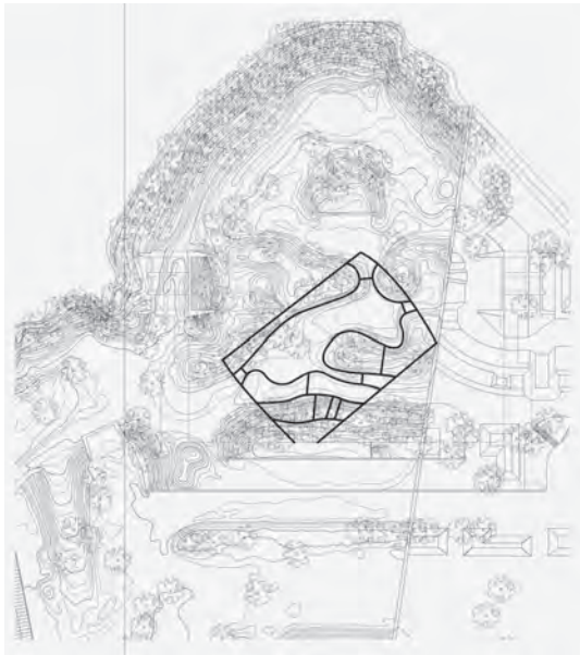
3a-c The trajectory of the curves during the design process: from contour lines on the plan given to the architect to poured concrete walls on the construction site.
