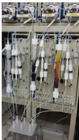
Figure 3.8: Test on food and feed samples with Jumbo method and 4 column set, from the left: blank, QC pork fat and commercial sunflower oil.
