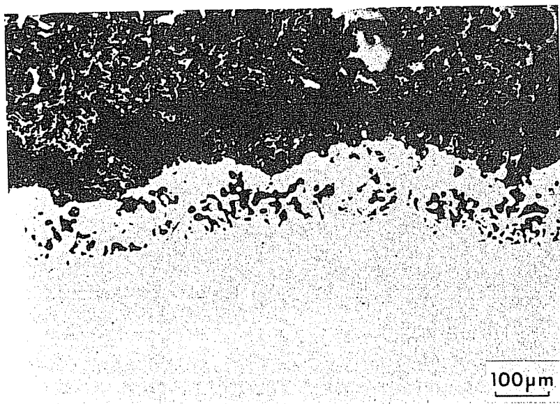
Fig. 3.28 Alloy E1 (Cu-Mn) after holding at 1200°C for 3 h. Unetched [10].
