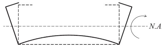
Figure 4.13 Flange curling of channel section beam
