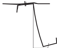
Figure 4.51 Distortion of purlin
