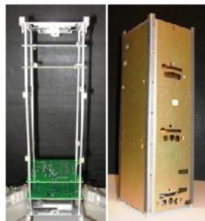
Figure 36 - Upper plate ( Left ), inside structure and solid chassis ( Right ) (Adapted from (DelfiSpace))
