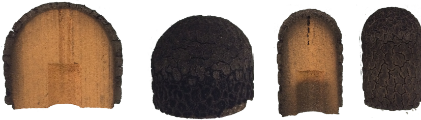
Figure 3.6.: Cross sections of Tests 14R (left) and 26 (right) with radii of 25 and 15 mm respectively. 11 mm samples were completely charred and could not be removed intact from the sample holder.
