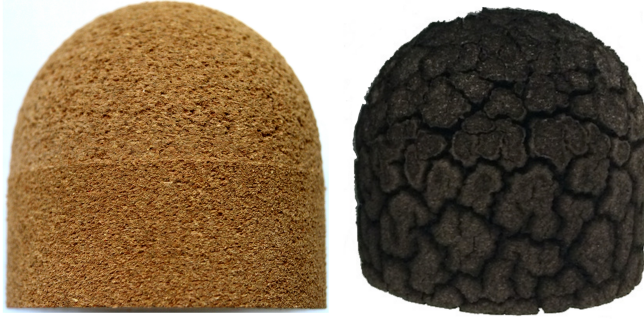
Figure 3.5.: Change of cork P50 surface topology from virgin (left) to char cracks (right) after Test 9R.
