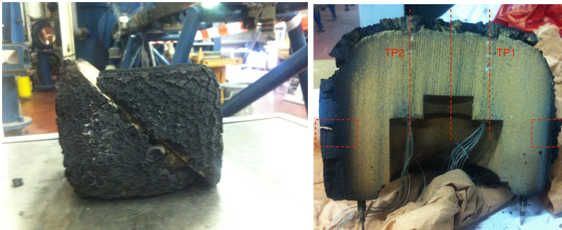
Figure 4.34.: Cork P50 cross sectioning for layers inspection.
