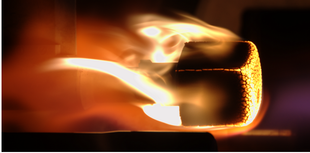
Figure 4.19.: Sample exposed to plasma. The thermal plug is at the lower right corner.
