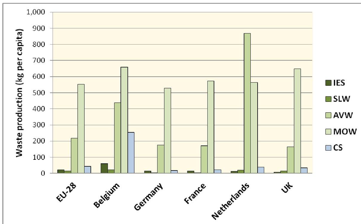
**Figure 5: Waste production in Belgium, Germany, France, the Netherlands and the United Kingdom in 2012 according to the type of waste expressed in kg per capita (non-hazardous wastes). The following wastes are considered: Industrial Effluent Sludges (IES), Sludges and Liquid Wastes from waste treatment (SLW), Animal and Vegetal wastes (AVW), Mixed Ordinary Wastes (MOW) and Common Sludges (CS).**
