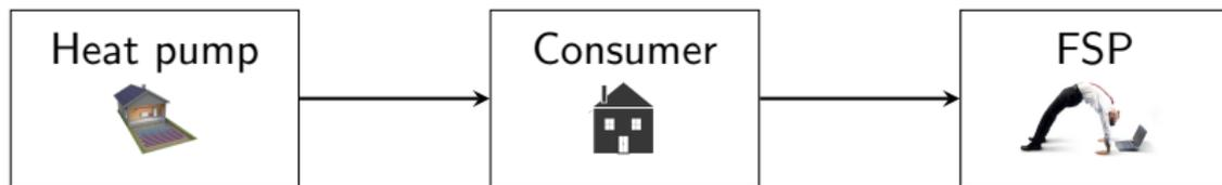
This **electrical energy** consumed by the heat pump is converted into **heat** which is **stored** by the **building** and, depending on its thermal inertia, allows consumption to be shifted.
