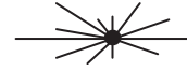
Figure 3: Hedgehog diagram (plane view) showing the intensities in norm and direction measured at a receiver's position.
