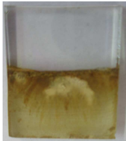
Figure 3.17: An FTO substrate coated 10 times with a solution of 0,25 M iron and yttrium, 0,5M citric acid with a pH adjusted to 4 mixed with a tipful of surfactant. Between the 5th and the 6th coating, the sample is heated at 300°C during 2h. After all the coating cycles, the sample is heated at 450°C for 2h.
