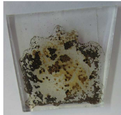
Figure 3.23: An FTOcG substrate covered with 3 drops of a solution of 0,25 M iron and yttrium, 0,5M citric acid with a pH adjusted to 4 mixed with a tipful of surfactant and heated at 500°C.
