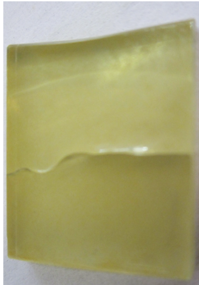
Figure 3.6: A broken glass substrate due to the thermal gradient.
