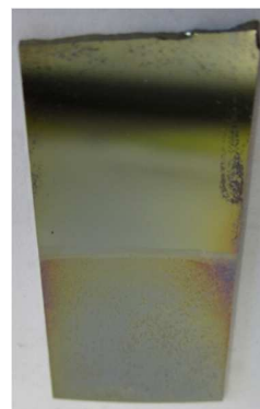
Figure 3.12: A Si substrate coated 2 times with a solution made of peptized precipitate. The sample is then heated at 450°C for 2h.
