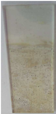
Figure 3.22: An FTOcP substrate coated 5 times with a solution of 0,25 M iron and yttrium, 0,5M citric acid with a pH adjusted to 4 mixed with a tipful of surfactant and heated at 850°C.
