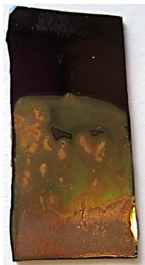
Figure 3.4: A sample where the inhomogeneous coating (more material is deposited at the bottom of the substrate) is mainly due to gravity.
