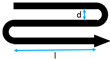
Figure 4.9: The spray line pattern with “ d ” the distance between 2 lines and “ l ” the length of the lines
