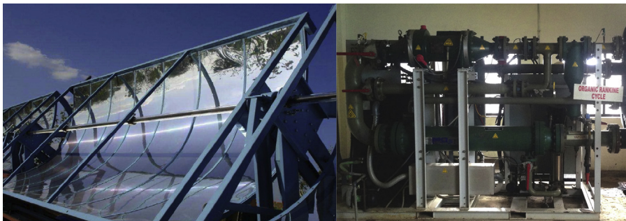
Figure 16.1 1 MW e Shive village electrification plant (Thermax India), a hybrid plant consisting of a concentrating solar power (CSP) collector field, steam Rankine cycle, Organic Rankine Cycle, and a backup biomass-fired boiler. Left: Thermax PTC collector. Right: GE/Calnetix 100 kW e ORC (Thakur, 2013).
