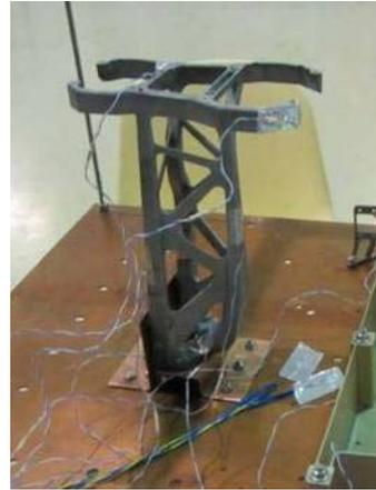
*Figure 8. Built part prepared for thermal cycling test*
