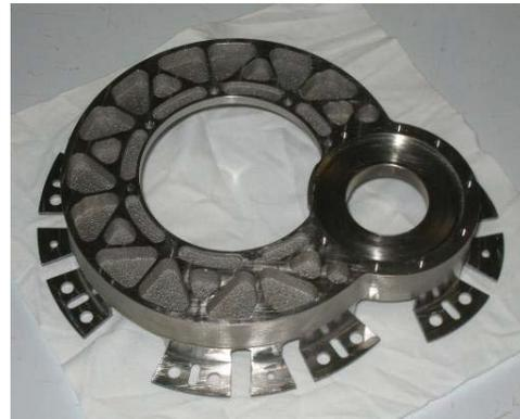
Figure 2. Final part manufactured by EBM
