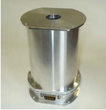
Figure 3. Reaction/Momentum Wheel Housing Assembly
