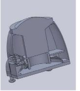
Figure 12. Cut view of the designed Sun Sensor
