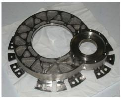
Figure 2. Final part manufactured by EBM
