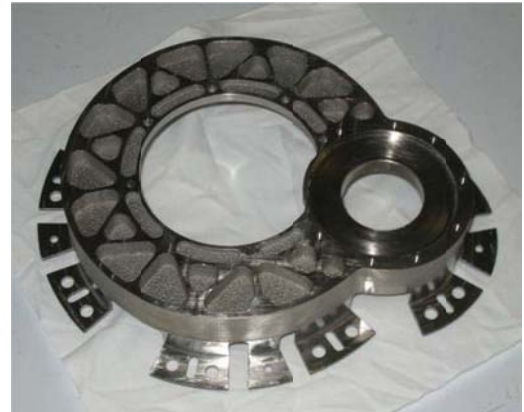
Fig. II: Final part manufactured by EBM
