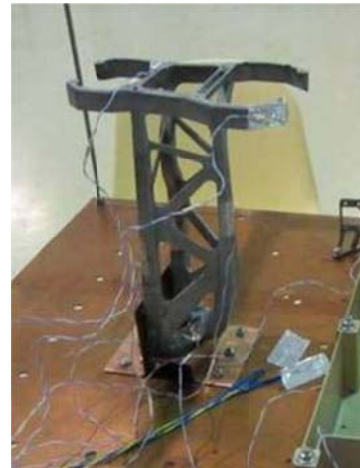
Fig. VIII: Built part prepared for thermal cycling test
