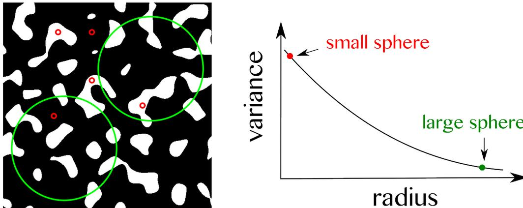
Figure 1. The scale-dependent heterogeneity of a material (left) can be characterized by throwing randomly spheres of radius  $R$  in it and counting the number of electrons they contain. This number is a random variable, the variance of which is a measure of the heterogeneity of the material at scale  $R$ .
