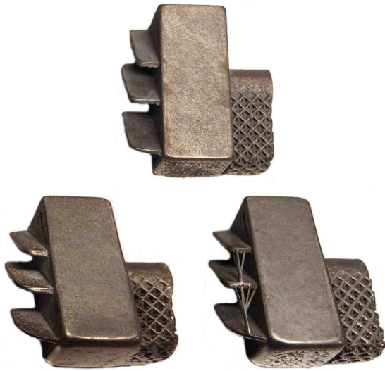
Fig. 12: Effect of the tribofinishing system on the samples treated for 60 minutes (top, SLMA) and 30 hours (bottom left, EBMT and bottom right, SLMT).
