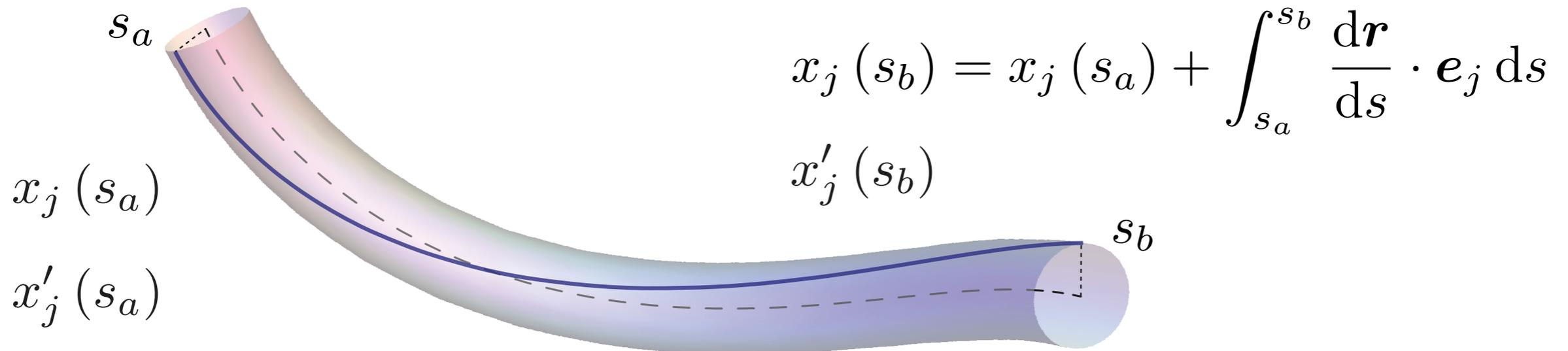
→ Integral constraints on the *unknown length*  $\ell = s_b - s_a$  of the rod
