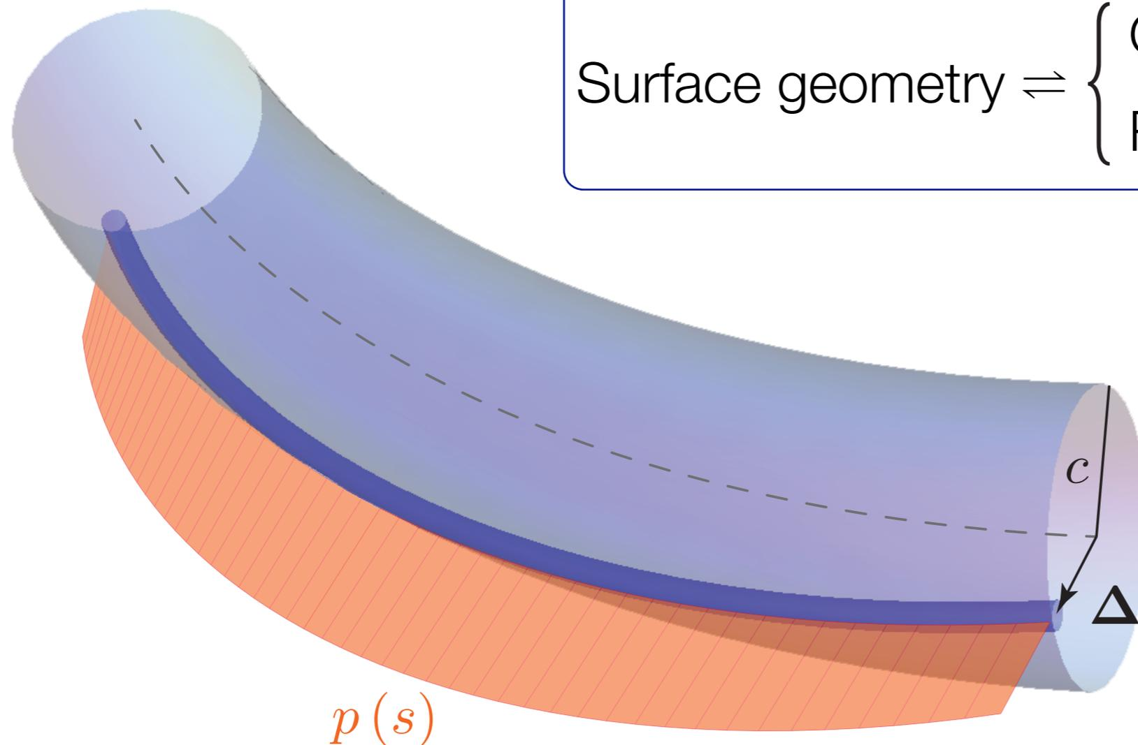
Surface geometry  $\Leftrightarrow$   $\begin{cases} \text{Contact geometry} \\ \text{Reaction pressure} \end{cases}$
