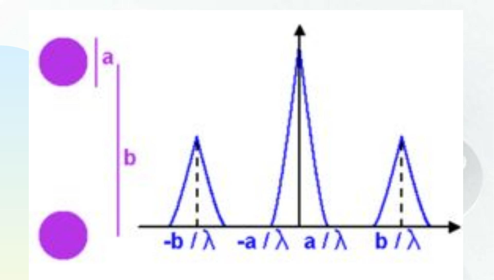
**Diagram illustrating the autocorrelation as a function of the space frequency, for the case of an interferometer composed of 2 telescopes, with a diameter  $a$ , separated by the baseline  $b$ . The autocorrelation of the pupil gives access to high space frequencies.**
