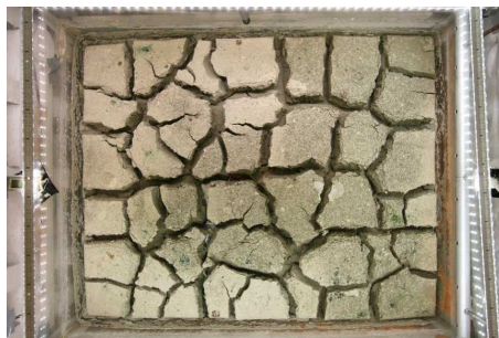
Fig. 2.10: Cracks network on the surface of the Romainville clay after drying (Ta, 2009).
