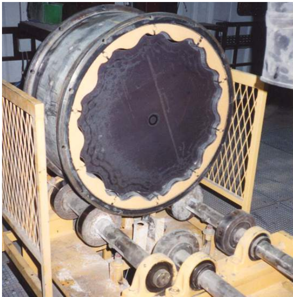
(a) Laboratory mill supported on driving shafts with a Duolift liner and closed by an end wall of tempered glass.
