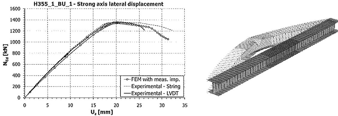
Figure 9: Experimental vs. numerical results for H355\_1\_BU\_1 test
