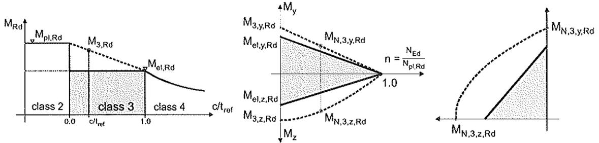
Figure 5: Illustration of the 3-step procedure (grey zones show the Class 3 resistances according to Eurocode 3)
