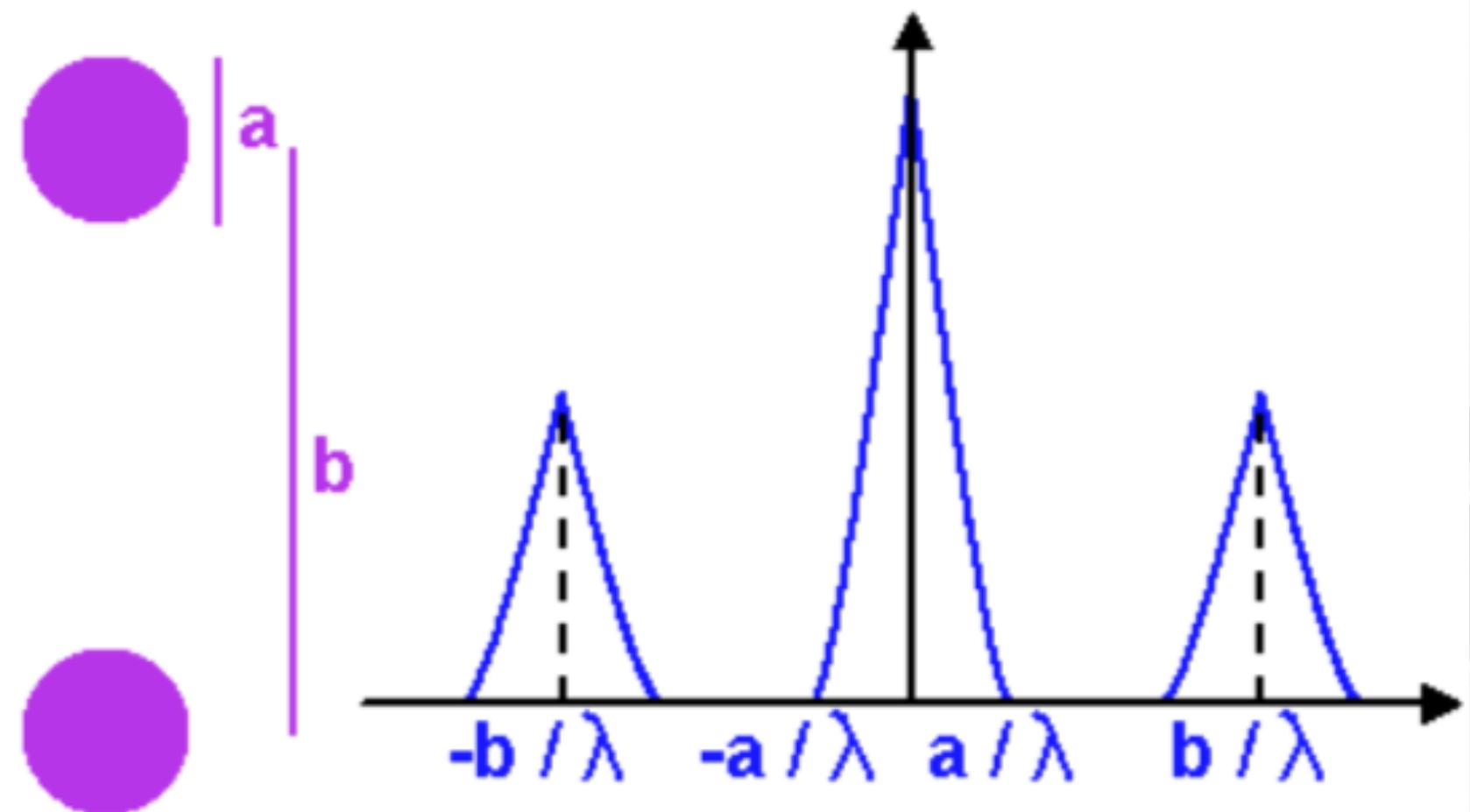
Diagram illustrating the autocorrelation as a function of the space frequency, for the case of an interferometer composed of 2 telescopes, with a diameter  $a$ , separated by the baseline  $b$ . The autocorrelation of the pupil gives access to high space frequencies.
