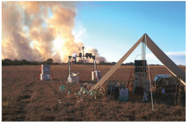
Figure 1.19 - Aerosol sampling set-up used during SAFARI 2000 in the Kruger National Park, South Africa. (W. Maenhaut, UGent-INW).
