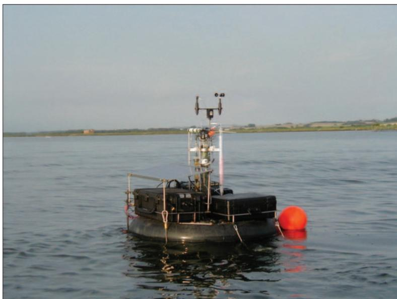
*Figure 3.3 - Floating Equilibrator System deployed in the Randers Fjord (Denmark). This device continuously monitors the CO<sub>2</sub> concentration of surface water, together with temperature, salinity, and meteorological parameters such as wind speed, air temperature, and solar irradiance. It is powered by batteries and a solar panel and includes an infrared spectrometer for CO<sub>2</sub> determinations. (ULg-OCEANCHEM).*
